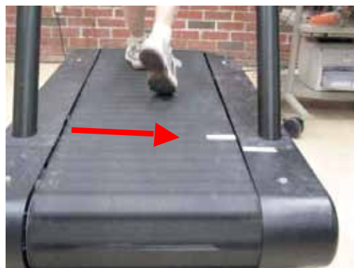
Figure B-2: Verifying the speed of the treadmill belt requires accurate timing of belt revolutions. Note that the tape mark on the belt is approaching the mark on the treadmill deck. Each pass of the tape on the belt counts as one revolution. See text for details. It is essential that an assistant walks on the treadmill while the belt speed is being verified.
