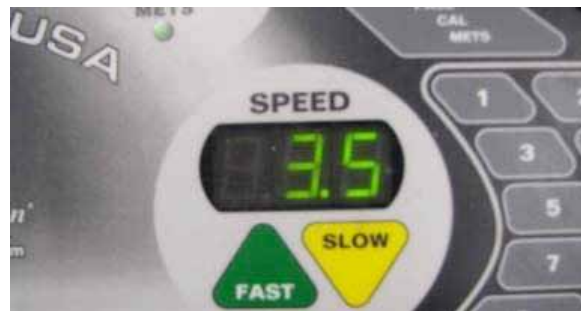
Figure B-1: Set controller to the desired speed
